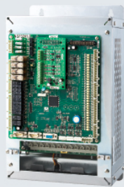
S8 Series Elevator Integrated Controller
